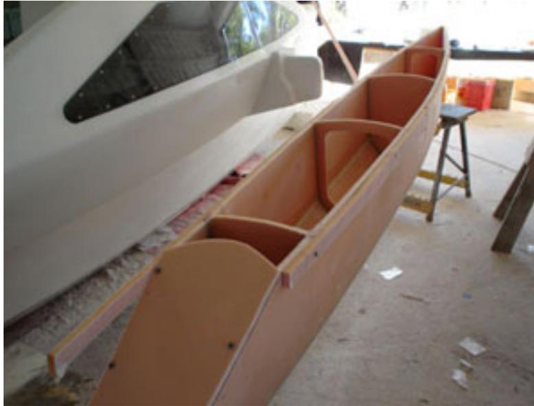
Doublers were added around the edge of the float to hold the deck.
