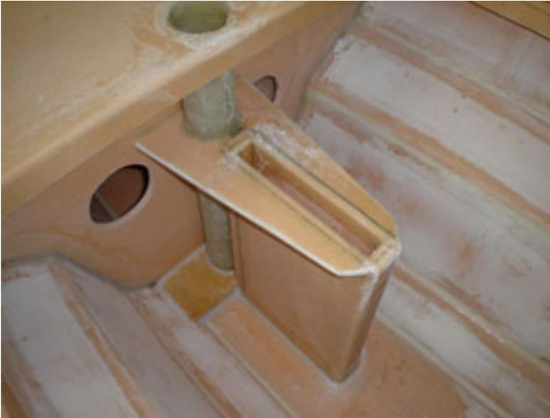
The inside of the hull was filled ready to paint.
