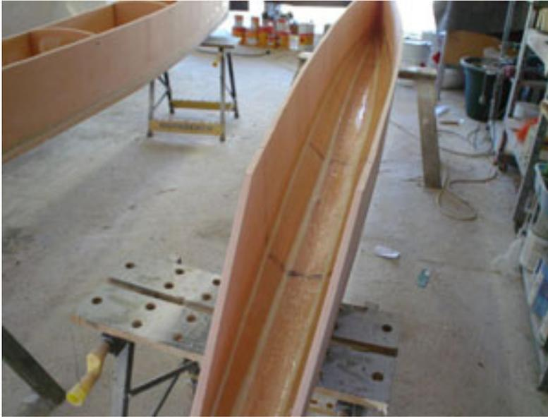
The float is levelled or you can use the markings that you added when attaching the panels. The bulkheads are added and taped in.
