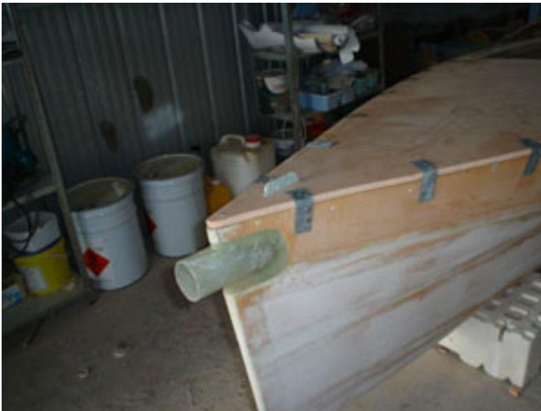
A plywood mast support was added and a hole cut in the hull bottom for the centreboard. The dagger-board case was made of laminated foam and taped to the floor.
