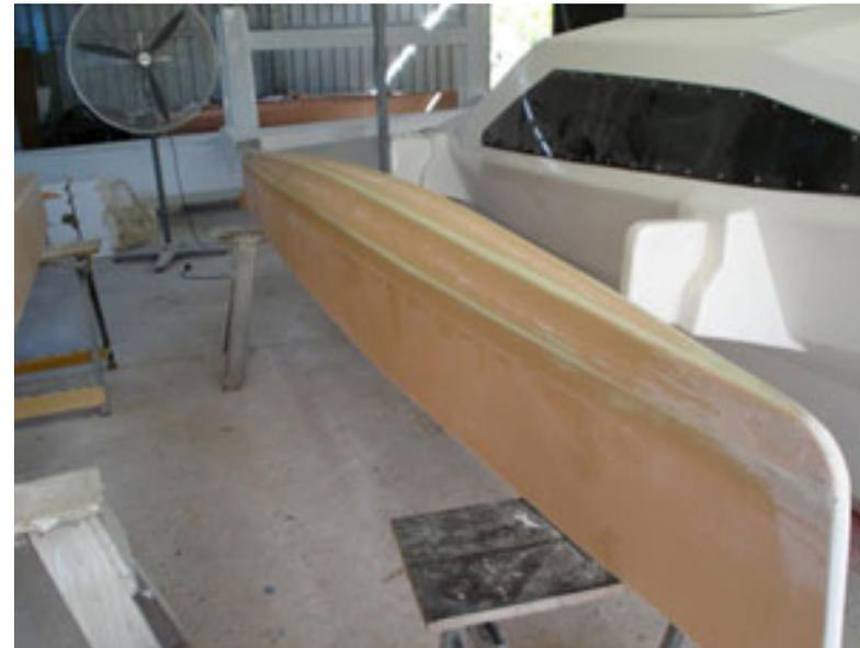
All the inside chines are taped using wet fillets.
